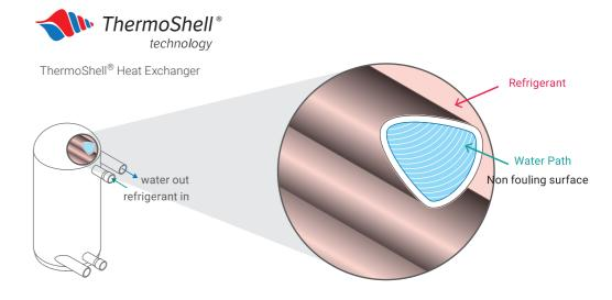
Coaxial Heat Exchanger
