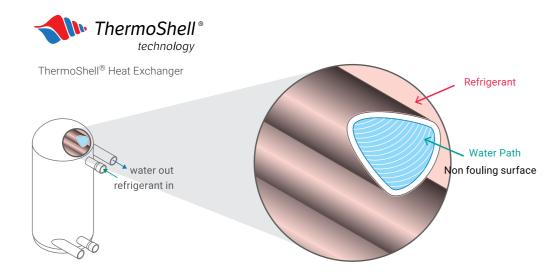
Coaxial Heat Exchanger
