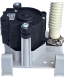
Drain Pumps Option Optional Condensate lift-pump (1m head) has been designed to remove condensate from the unit in tight installations where a well sloped drain line (minimum 1 in 50 gradient) is not feasible.
