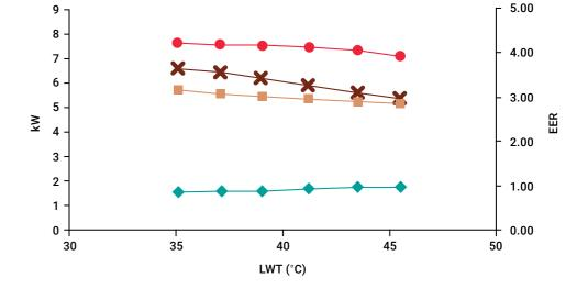
A 5°C increase in LWT results in water flow rates down from 0.36 l/s to 0.18 l/s
