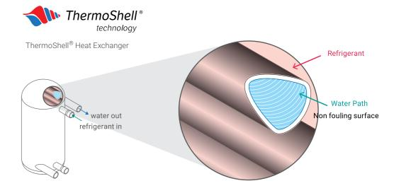
Coaxial Heat Exchanger
