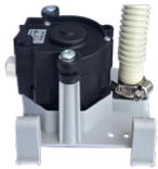
Drain Pumps Option Optional Condensate lift-pump (1m head) has been designed to remove condensate from the unit in tight installations where a well sloped drain line (minimum 1 in 50 gradient) is not feasible.
