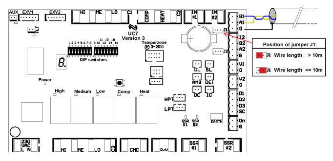
Up to a maximum of 99 units can be connected on a common RS485 bus in daisy-chain fashion.
