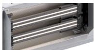
PTC Electric Heat Option All HWP electric heat units feature Positive Temperature Co-efficient (PTC) elements, which adapts its output relative to air velocity. Due to this surface temperature control these safe self-limiting elements will not overheat.
