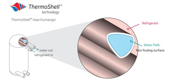
Coaxial Heat Exchanger
