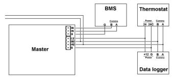
Temperzone has available a low cost data logger specifically designed for use with temperzone units. The Temperzone data logger connects to the same terminals as a communicating thermostat. The Data logger connections are shown above. Note that a BMS, communication thermostat and data logger are all optional and can be omitted or added as desired. The UC7 controller automatically configures itself when power is applied to the unit.
