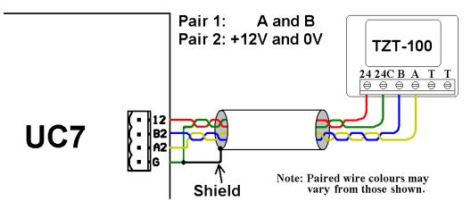
The TZT-100 thermostat can also be powered by an **isolated** 24V AC power source as shown below:
