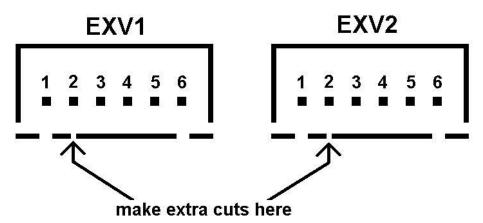
DIP switches 7 and 8 on UC7 board define how the outputs EXV1 and EXV2 are operated. Refer to section 4 (DIP switch selections) for more details.
