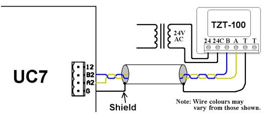
In this case the 24V AC supply common should NOT be earthed elsewhere in the system, otherwise differences in earth potentials can lead to unreliable communications between the thermostat and the UC7.
