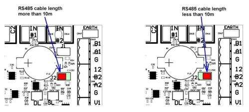
If the distance between the thermostat and the UC7 is greater than 10m and the UC7 is located at one end of the cable then place jumper "J2" on the centre and left pins
