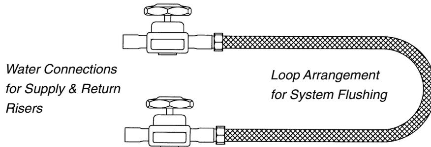
3. Open the air vents and fill the system with clean water. Monitor that the air vents do not overflow.
