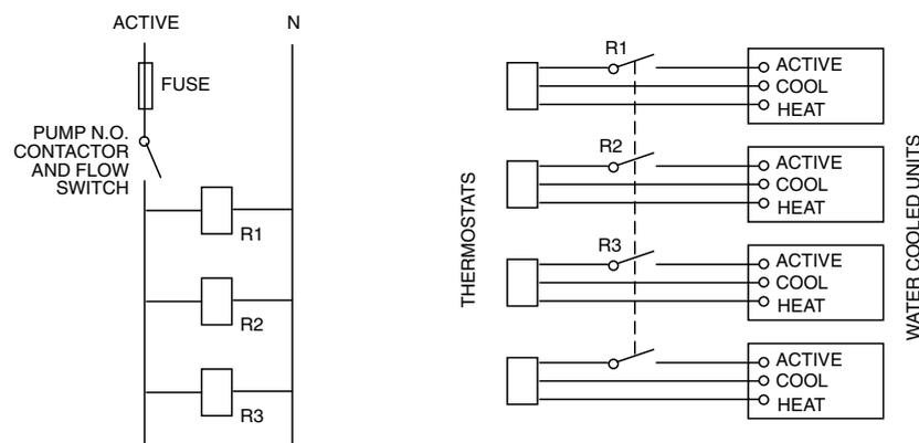
**Typical Single Relay Set-Up**
