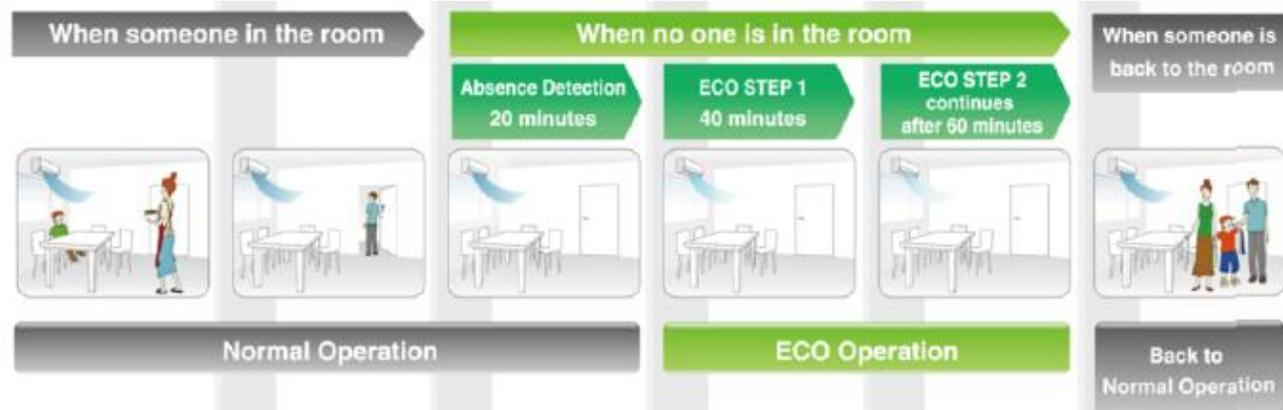
When nobody is detected in the room, the energy saving operation will start automatically in 2 steps.
